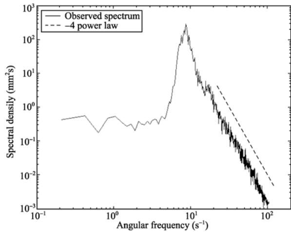
Fig.1 A typical wind wave spectrum observed at Physical Oceanography Laboratory's wind-wave-current flume in the Ocean University of China. The wind speed, fetch and significant wave height are  $10\text{ m s}^{-1}$ , 40m and 0.061 m, respectively.
