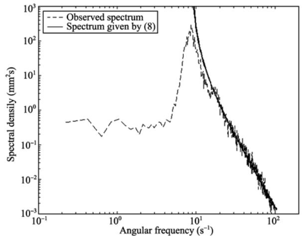
Fig.2 Spectrum expressed in (8) and the observed spectrum.  $\omega_0$  in (8) is chosen as the peak frequency of the observed spectrum, i.e.,  $\omega_0 = 8.6 \text{ s}^{-1}$ . The parameters of the observed spectrum are the same as those in Fig.1.
