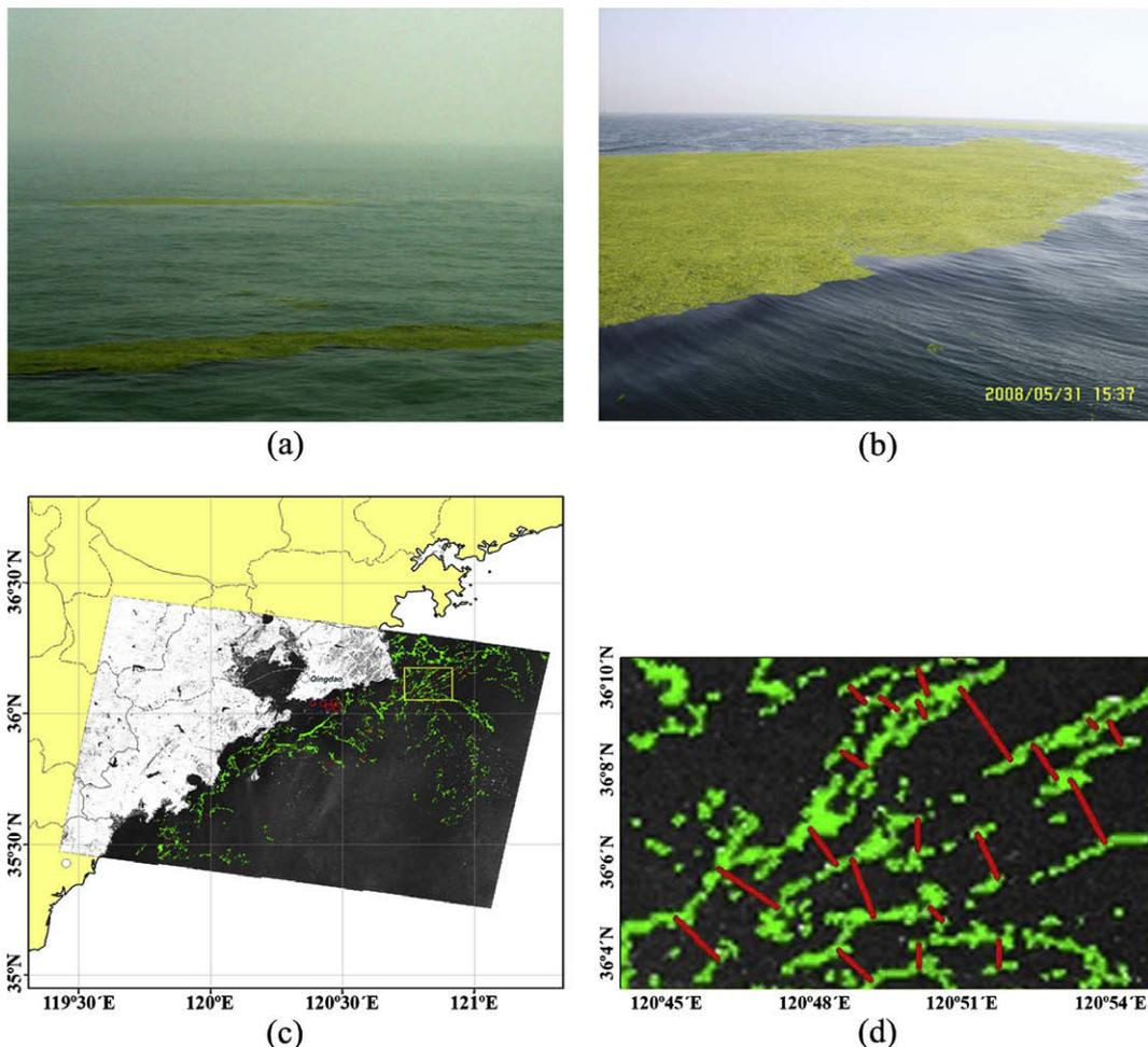
**Fig. 2.** The banded structure of the drifting macroalgae on the sea surface. (a) A photograph from a surface vessel on July 6, 2008 at (36°00'18"N, 120°29'48"E). The two bands of macroalgae are about 400 m apart; (b) a photograph taken from an aircraft at 15:37, May 31, 2008 off Qingdao. The width of macroalgae band is about 30 m; (c) SAR images of the macroalgae obtained from COSMO-2 on July 13, 2008; (d) subfigure magnified from the part of figure (c) enclosed by the yellow rectangle.
